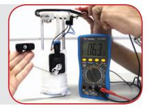
**3-** Adjust the multimeter to the resistance scale (Ohm);
