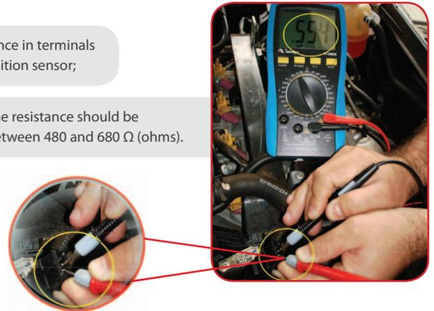
**Note:** Each injection system is provided with a crankshaft position sensor with a specific resistance value, which varies pursuant to the gauge and the number of turns of the coil.
