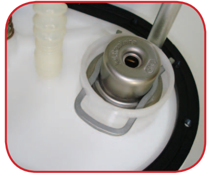
In the fuel module, next to the fuel pump (returnless multi-point system).
