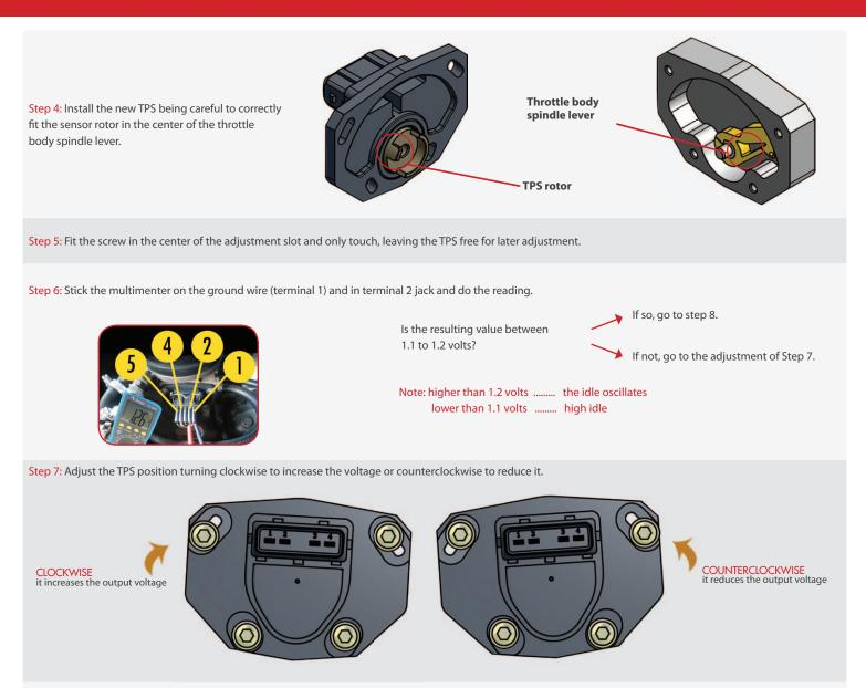
Step 8: When the position is right, tighten the screws.
