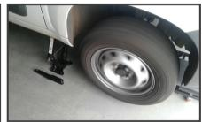
Lift the two front wheels. Start engine and engage 3rd level shift (when not using an elevator, leave a person inside the car for safety)
