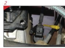
2nd Analyze Signal of Sensor To analyze the signal, you can use an oscilloscope or a Hertz frequency scale (Hz) automotive multimeter conferring the signal generated on pins B and C.
