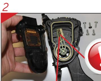
Remove the lid very carefully, keeping the knuckle contact;
