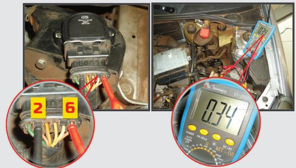
**Step 8:** Keep the part position and check pins 2 and 5. The voltage obtained should be 0.70 ( $\pm 0.05$  volts), in other words, it should double pin 6;
