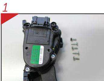
Remove the set screws from the lid very carefully in order to avoid damage to the contact pads that connect with the card;
