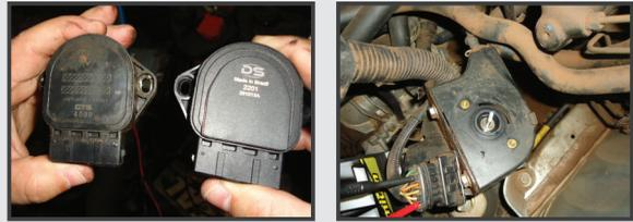
**Step 7:** Adjust the multimeter at the continuous voltage scale (20 V) and check pins 2 and 6. The voltage obtained should be 0.35 ( $\pm 0.05$  volts). If not, spin the part in the device until you get the correct reading;
