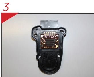
Remove the damaged card;
